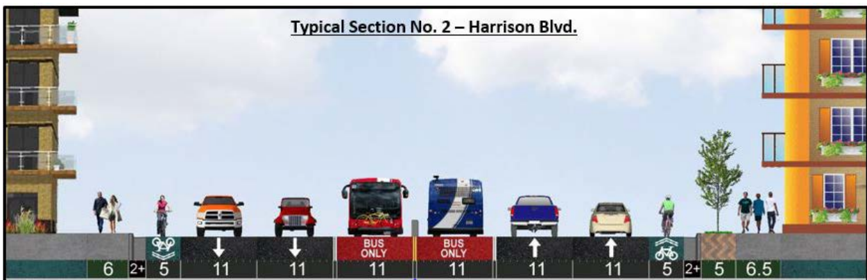
Figure 12. Cross-section of Roadway on Harrison Boulevard
