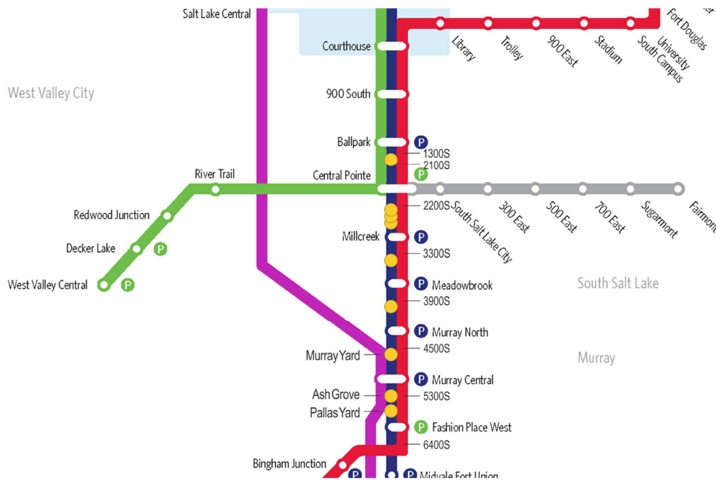
Figure 38 – North/South Line Active Freight Switches (Shown as Yellow Dots)
