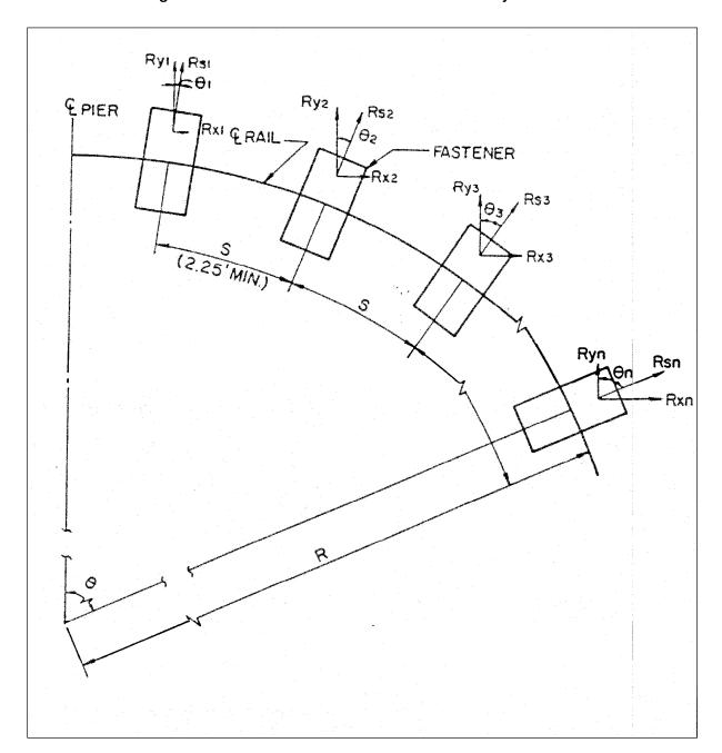
Figure 7-8: Lateral Restraint of Transverse Force by Fastener
