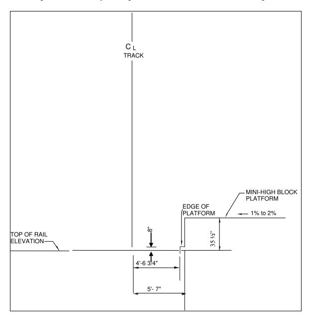
Figure 3-4b: LRV Only Mini-High Block Platform Minimum Clearance Diagram
