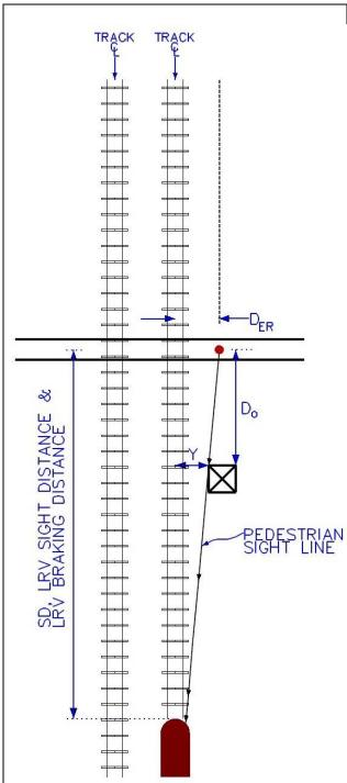
Figure 19-4: Application of Pedestrian Safety Treatments (From the UDOT Pedestrian Grade Crossing Manual)
