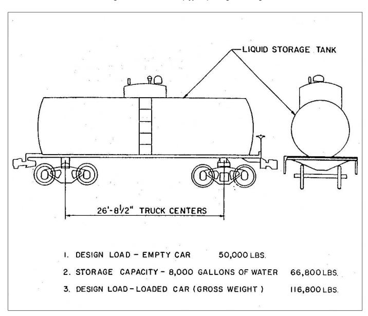
Figure 7-6: Work Train (Type C) Design Loading
