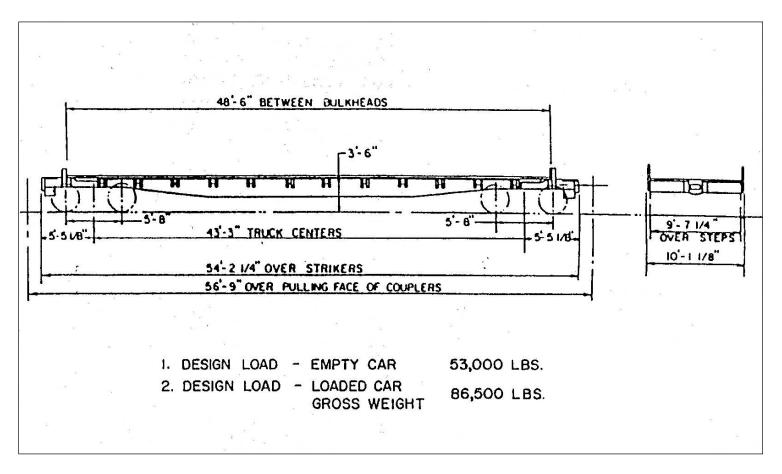
Figure 7-4: Work Train (Type A) Design Loading
