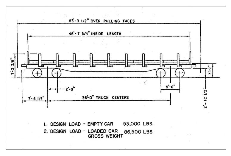
Figure 7-5: Work Train (Type B) Design Loading
