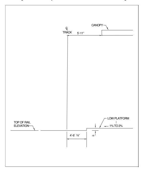
Figure 3-3b: LRV Only Low-Center Platform Minimum Clearance Diagram
