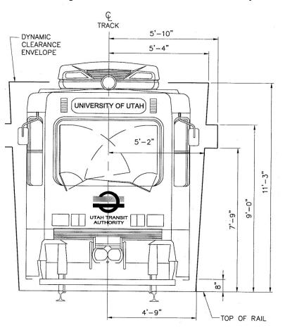
Figure 3-1: CLRV Static Dimensions and Dynamic Outline (Tangent Track)
