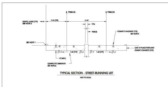
Figure 4-2a: Typical Section of Street-Running LRT
