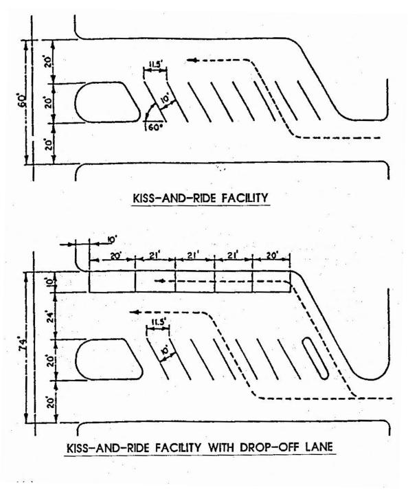
Figure 20-3: Kiss-and-Ride Parking Arrangement Stall Layout 60°
