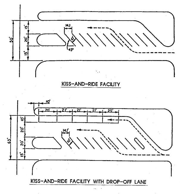
Figure 20-2: Kiss-and-Ride Parking Arrangement Stall Layout 45°
